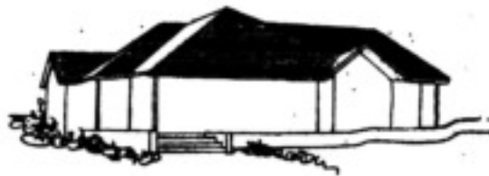
Hipped Roof with Gables
